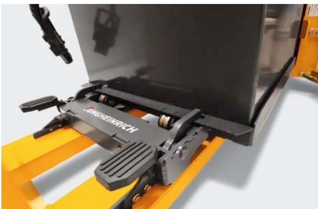
Two side foot notches to open/close the connection with the battery trolley.
