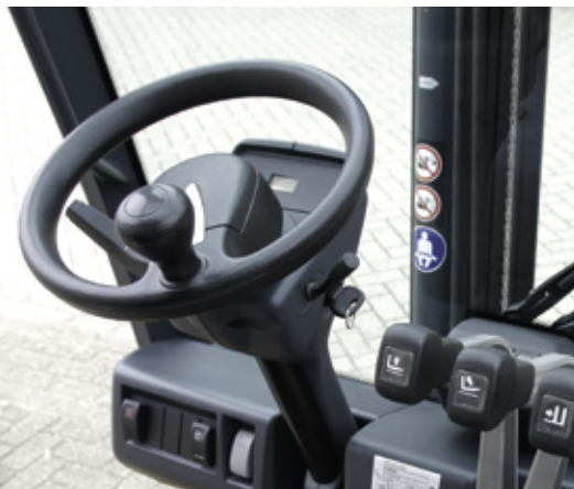
04 The slim steering column (with the travel direction lever on its left side) is infinitely variable
