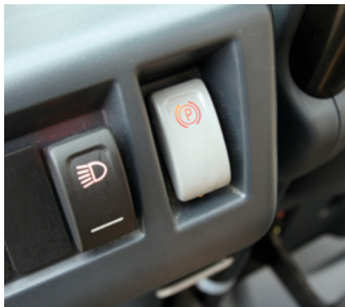
05 The grey switch activates the electrical wheel stop of the maintenance-free brake system
