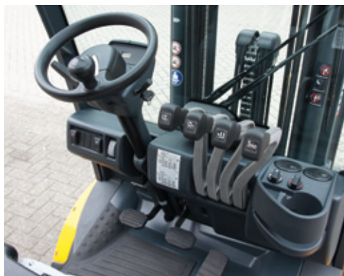
02 There is sufficient space available to comfortably operate the pedals, crawl speed and brake as well as the accelerator
