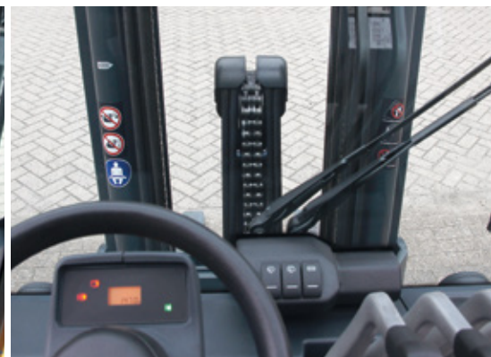
03 Visibility through the triplex mast is very good. The cylinders, chains and hoses have been positioned to optimise visibility
