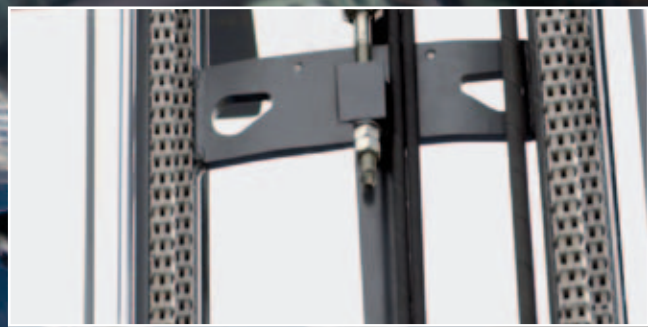
Viewing windows in the cross member ensure a clear view of the fork tips.
